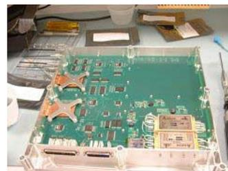
**Figure 10-** Real time image compression system GEZGIN
