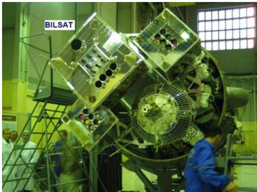
**Figure 1- On the launch vehicle:** All DMC satellites as well as other payloads are on the launch vehicle and ready for launch. BILSAT-1 satellite took place on the top to be released first once the upper most stage was in orbit.
