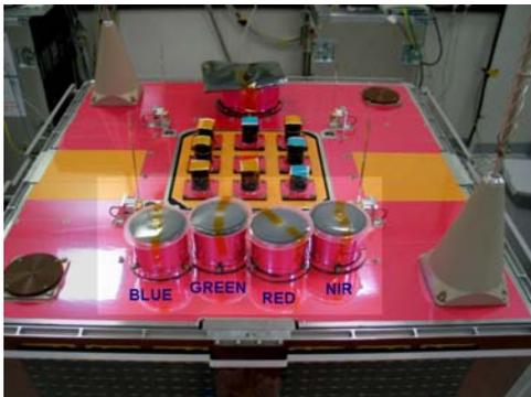
**Figure 5- Multi spectral imaging system channels on the earth facing facet:** Four channels exist in the blue, green, red and NIR (left to right) order. In this picture, temporary caps are closed to protect the lenses against any dust, dirt etc
