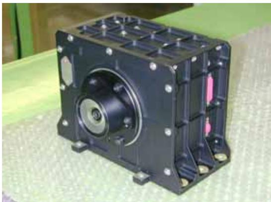
**Figure 22. CCD Earth Sensor Assembly (CCDESA)**
