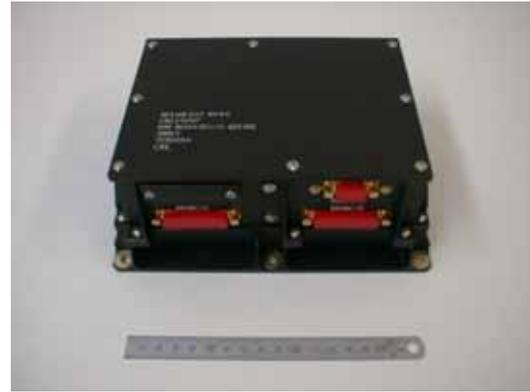
**Figure 12. On-board image processing microprocessor module (MOBC)**
