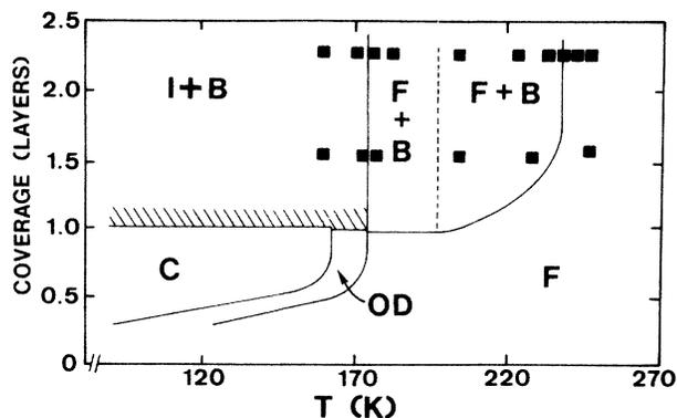
FIG. 1. Proposed phase diagram for  $\text{Fe}(\text{CO})_5$  on graphite. Squares correspond to x-ray diffraction scans. See text for definition of the phases. Dashed line indicates onset of fluid monolayer-to-bilayer transition.
