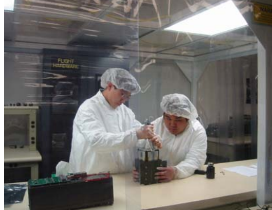
Figure 14: South Korea's CubeSat, HAUSAT-1, is removed from the test pod to proceed with the fit-check.
