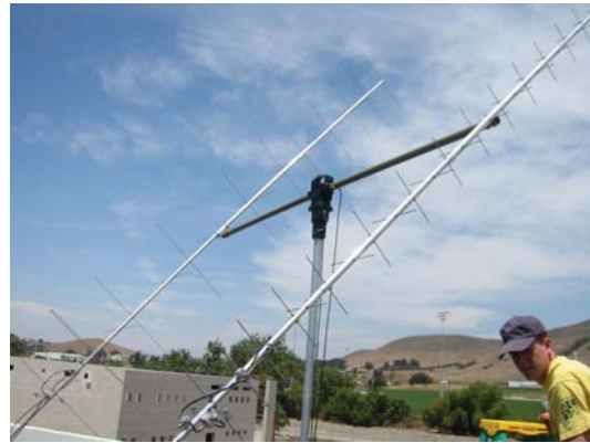
Figure 15: 2, 20 feet Yagis antennas provide high gain and directional pointing for satellites.
