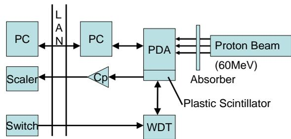
Figure 6 Radiation Test Setup Block Diagram
