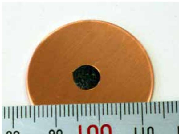
**Figure 4 Prototype of Electron Emitter**
