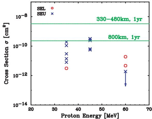
Figure 9 Cross Section for PDA
