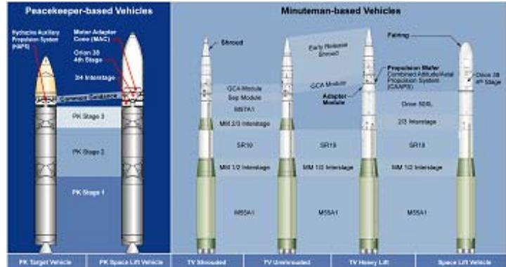
**Figure 1: RSLP Launch Configurations**
