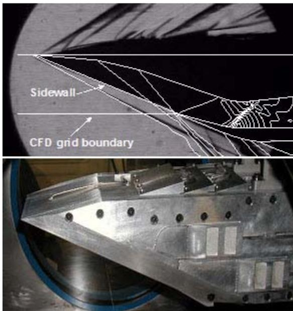
**Figure 8. High-Speed (Mach 2.5) Schlieren Image with Superimposed CFD Shock Train Demonstrating a Successful Self-Start (top), and the Sub-Scale Inlet Model in the Tri-Sonic Wind Tunnel (bottom)**
