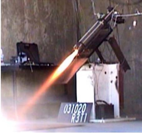
**Figure10. Sub-Scale Motor Testing to Acquire Burn Rate Data for the Design of the Heavy Weight Hybrid Rocket Motor**
