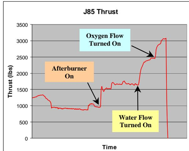
**Figure 6. Thrust Profile for the J85 Engine with the Addition of MIPCC (Inlet Condition:  $M=1.7$  at 40kft)**
