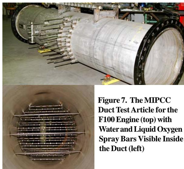
**Figure 7. The MIPCC Duct Test Article for the F100 Engine (top) with Water and Liquid Oxygen Spray Bars Visible Inside the Duct (left)**
