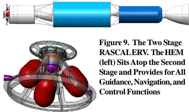
**Figure 9. The Two Stage RASCALERV. The HEM (left) Sits Atop the Second Stage and Provides for All Guidance, Navigation, and Control Functions**
