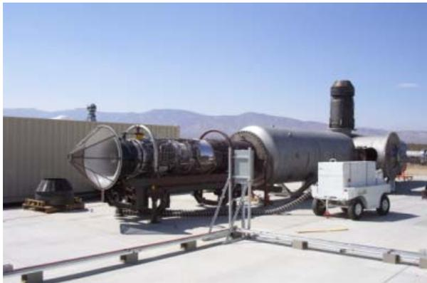
**Figure 5. J79 Source Engine Feeding into the Plenum at the MIPCC Test Bench in Mojave**
