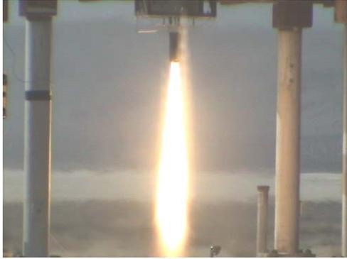
**Figure 10. Initial LOX/Propylene Static Fire Test**
