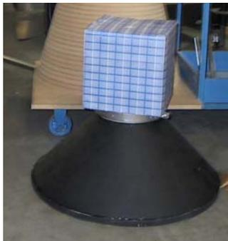
**Figure 5. Initial Mockup of Payload, Payload Adapter and 9-in. Attachment Clamp**
