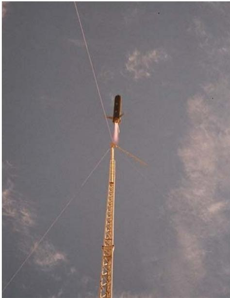
**Figure 8. Second Flight Test of a Liquid-Propellant Aerospike Engine on the First Launch of the Prospector 4** (photo by K. Caviezel)
