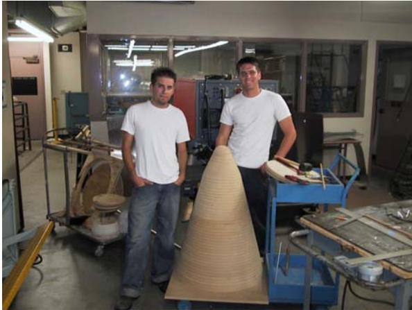
**Figure 4. CSULB Students with Fairing Lay-up Plug**
