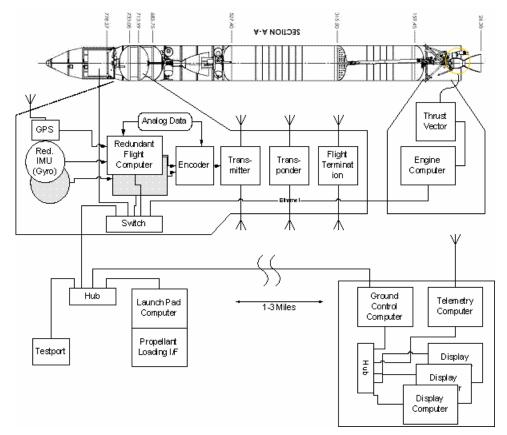
Figure 5: Avionics Architecture
