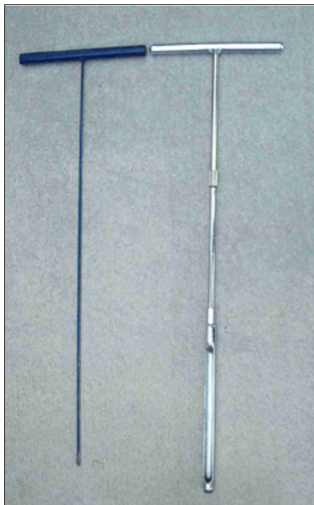
A tile probe (left) and soil probe (right)
