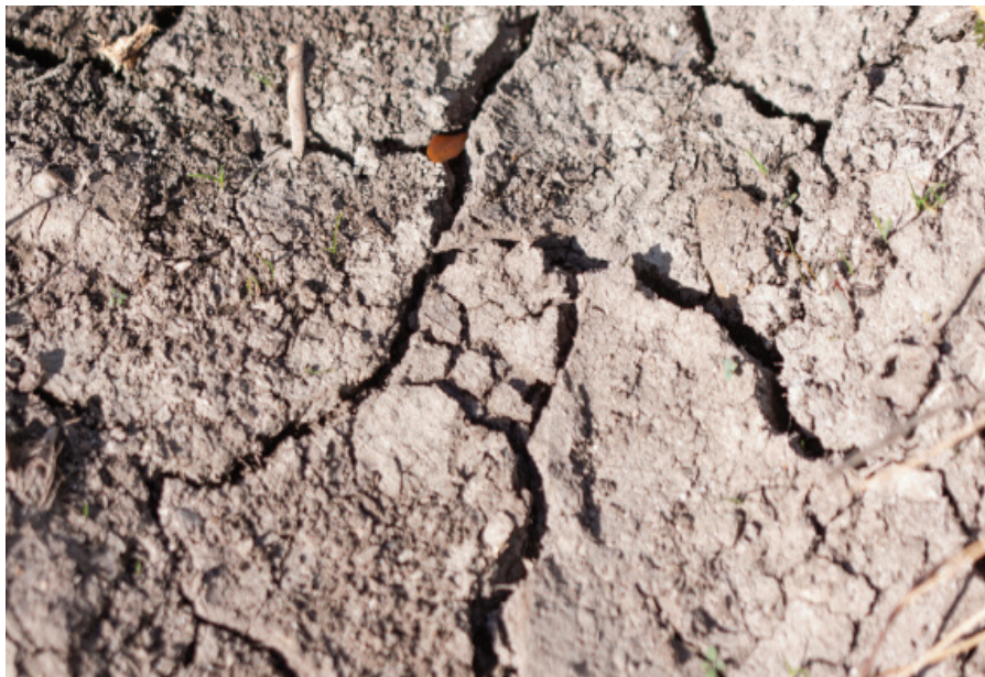
Clay soils may form cracks or crusts as seen in this soil located at a construction site.
