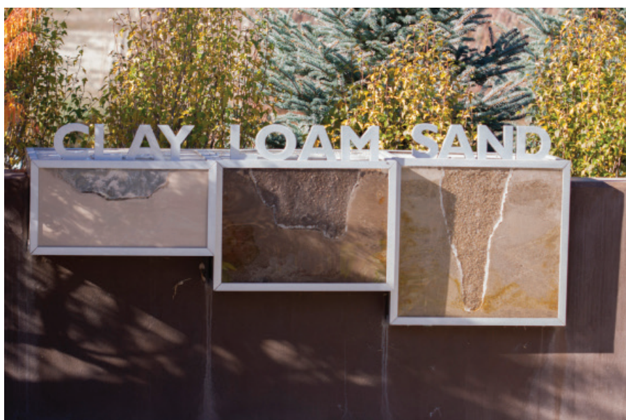
This educational display at Jordan Valley Conservation Garden Park in Salt Lake County shows water movement through clay, loam, and sandy soils.
