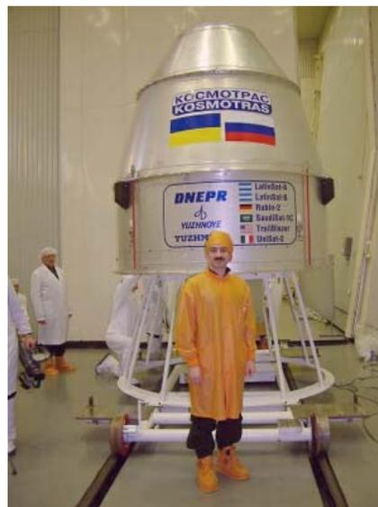
Fig. 9 Dnepr Payload Encapsulation Module
