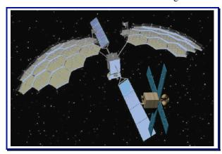
Figure 3. SCOUT-Based Escort Inspecting a Primary Satellite.
