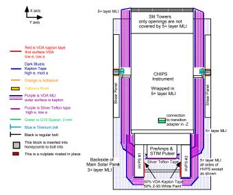
Figure 9: CHIPS Instrument External Thermal Design (+Z View)
