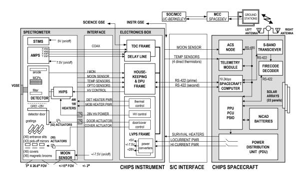
Figure 4: CHIPS Electrical System Block Diagram.
