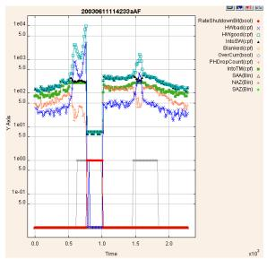
Figure 5: HVPS autonomous shutdown on orbit.
