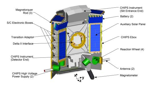
Figure 6: CHIPSat Rendering.
