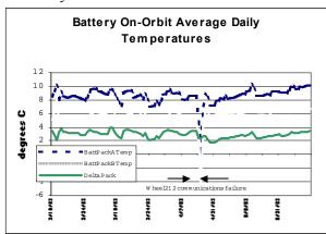
Figure 8: CHIPSat Battery On-Orbit Temperature Results
