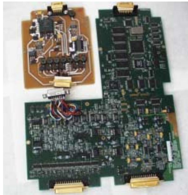
*Figure 7: MOST Instrument Computer*
