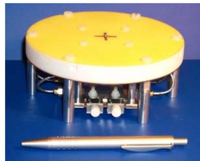
Figure 3 X band antenna
