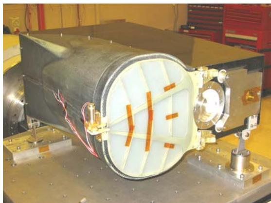
Figure 7 Camera flight structure qualification
