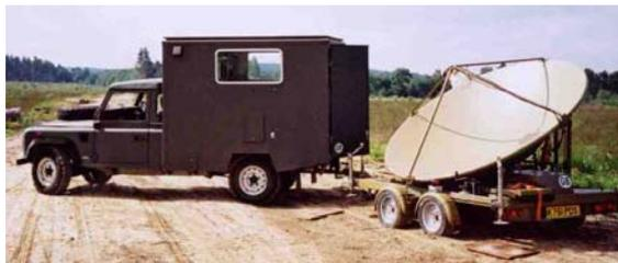
Figure 6 Mobile ground station,
