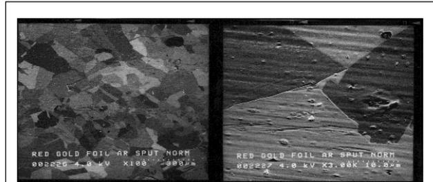
**Fig. 2** SEM image of Ar sputtered polycrystalline Au.
