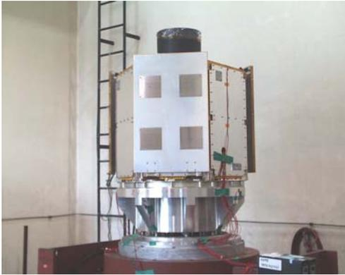
Figure 7. Vibration Test of SM/EOS
