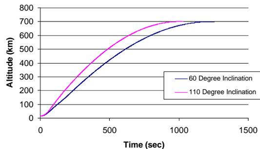
Figure 6. Altitude vs. Time for Chimera.
