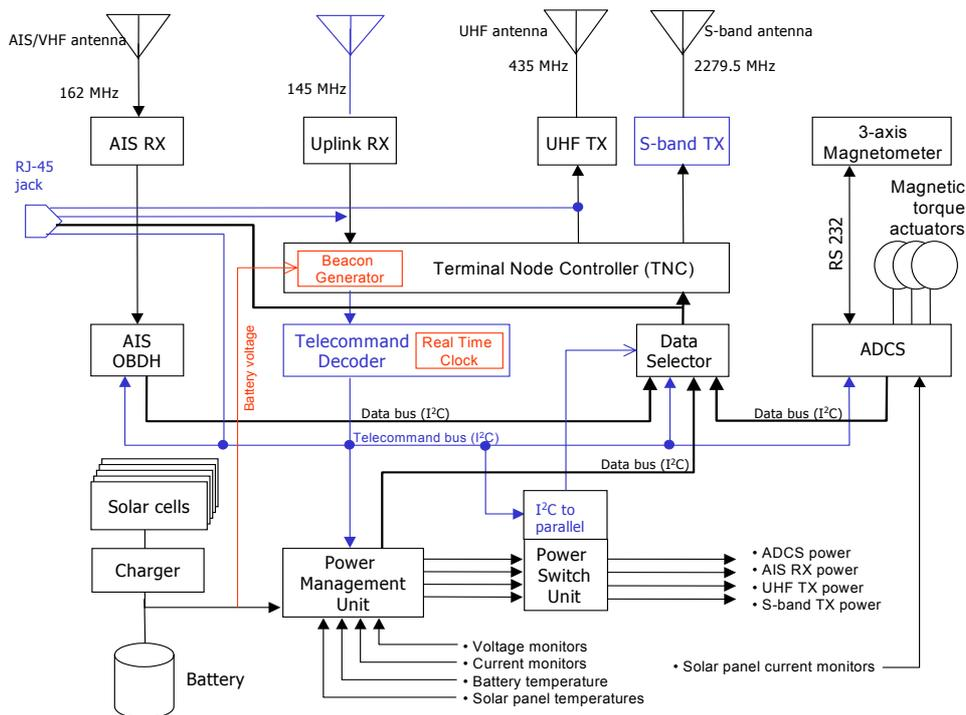
Figure 2. Satellite system architecture.
