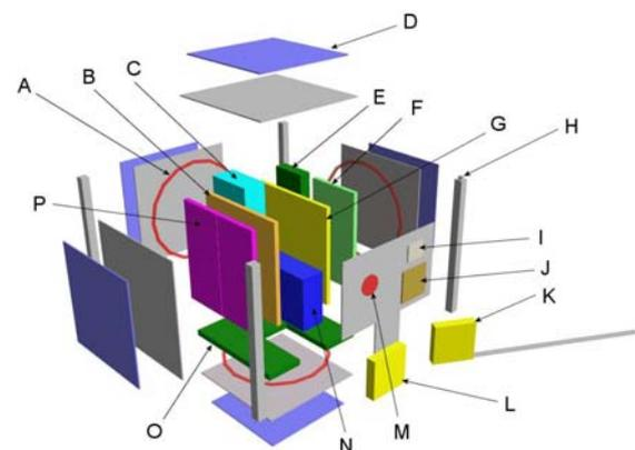
Figure 1. Exploded view of nCube subsystems
