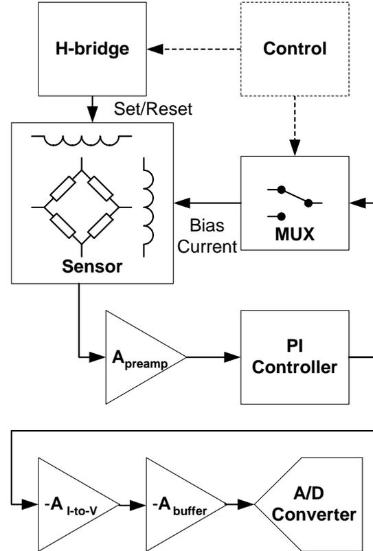
Figure 3: Block diagram of the magnetometer HW.
