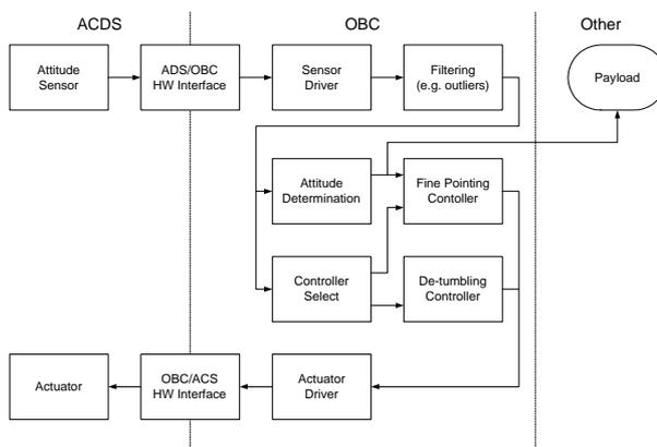
Figure 2: Block diagram of the DTUosat ACDS.
