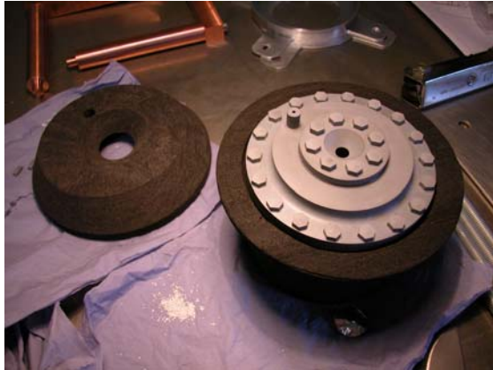
Figure 23. Solar receiver in graphite insulation package (cap section removed).
