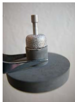
Figure 12. Braze test specimen, Mo/Ru filler, Mo cap, IMC post. Pressure < 10^{-4} mbar.
