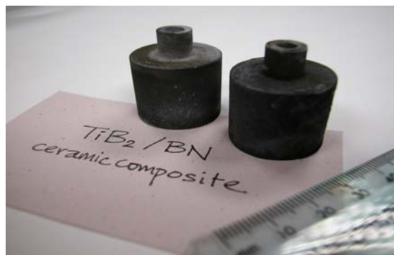
Figure 6. Post-test samples of IMC ceramic composite, 40 minutes at 2,300 K, 20 mbar He environment, graphite furnace.
