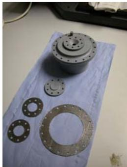
Figure 8. Solar receiver and graphite foil (Grafoil) gaskets.
