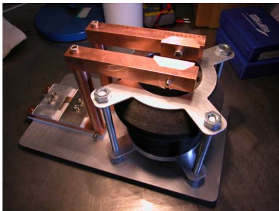
Figure 24. Solar receiver heating test rig. Copper electrodes are suspended over the receiver aperture; the heating element is clamped between the electrodes and inserted inside the cavity.
