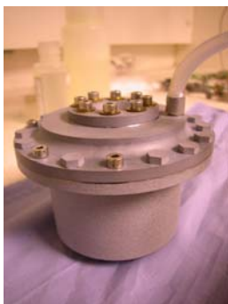
Figure 9. Sealed solar receiver undergoing 3.9 bar leak check.
