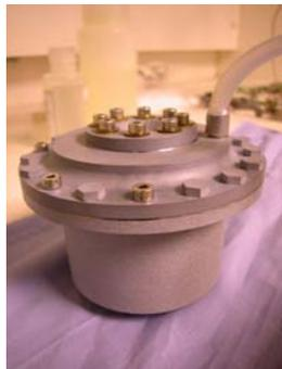
Figure 9. Sealed solar receiver undergoing 3.9 bar leak check.
