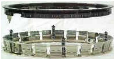
**Figure 3** Lightband® Separation System [5]
