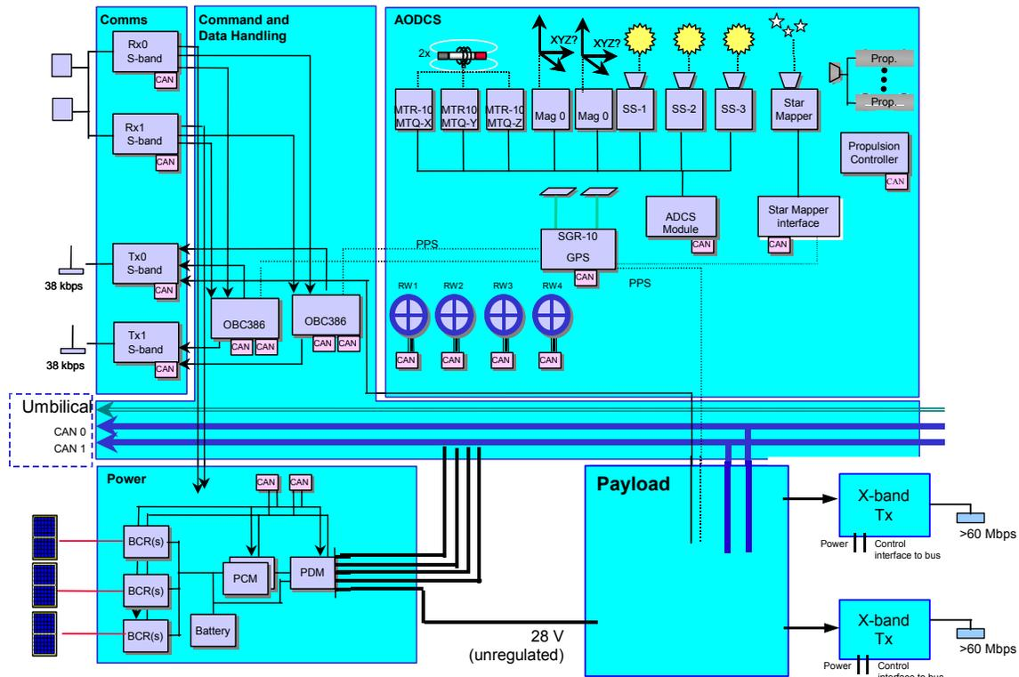
Figure 3 Spacecraft Block Diagram and Architecture
