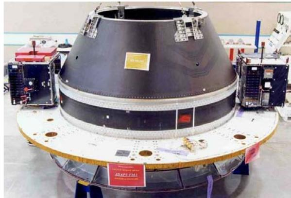
**Figure 2. QinetiQ STRV microsattellites mounted on the Ariane-5 ASAP destined for GTO**
