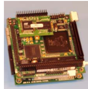
Figure 5 – Baseline flight computer in PC/104 format.
