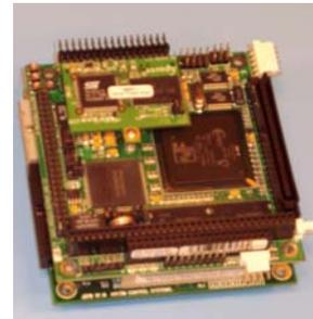
**Figure 5** – Baseline flight computer in PC/104 format.
