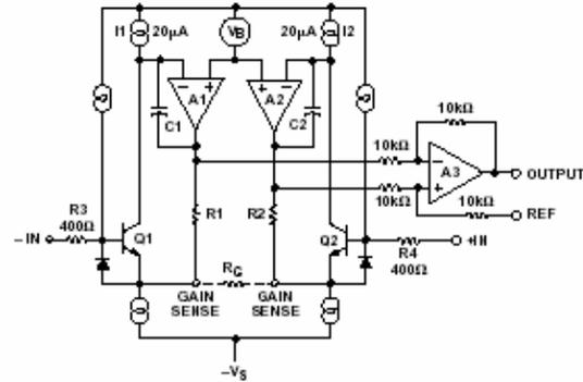
Figure 9. Instrumentation Amplifier Simplified Schematic<sup>11</sup>
