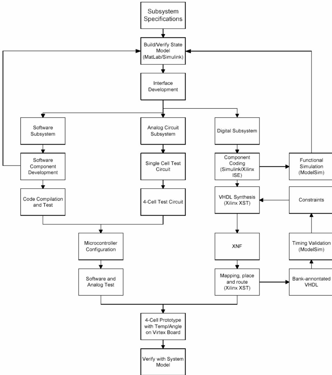
**Figure 5. Development Board Design Flow<sup>3</sup>**
