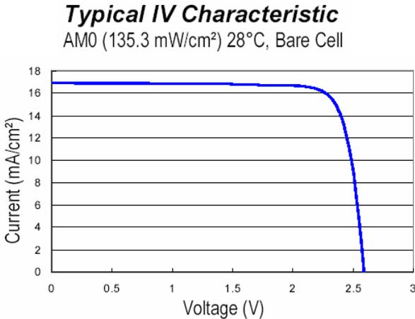
**Figure 3. Triple Junction Cell Typical IV Curve**
