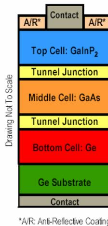
Figure 2. Triple Junction Solar Cell Layer Diagram and Electrical Model<sup>1</sup>
