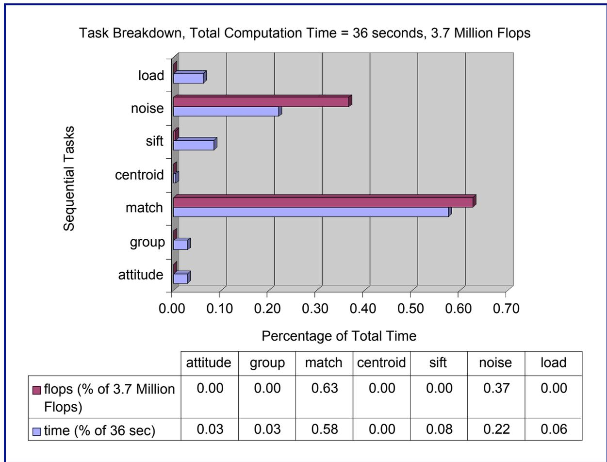
**Figure 7. Computation Requirements of each Task in Time and Flops.**
