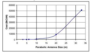
Figure 3: Parabolic Antenna Size vs. Cost
