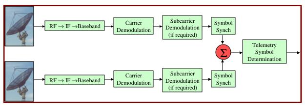
Figure 6: Symbol Stream Combining Block Diagram
