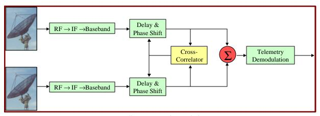
Figure 7: Full Spectrum Combining Block Diagram
