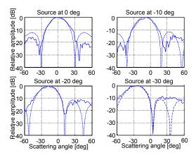
Fig. 10. Example of a bistatic RCS measurement [7]. These plots show the bistatic patterns when the RF source signal is incident at 0°, -10°, -20°, and -30°.
