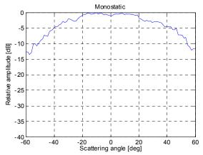
Fig. 9. Example of a monostatic RCS pattern [7].
