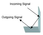
Fig. 2: Two-sided corner reflector, in which an incident signal reflects off both faces and back in the direction of the incoming signal.
