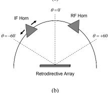
Fig 8. A retrodirective signal is characterized by (a) monostatic RCS and (b) bistatic RCS measurements.
