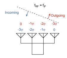
Fig. 3: Four-element Van Atta array. Retrodirection is achieved since the phase progression of the incoming signal is opposite to that of the outgoing signal.
