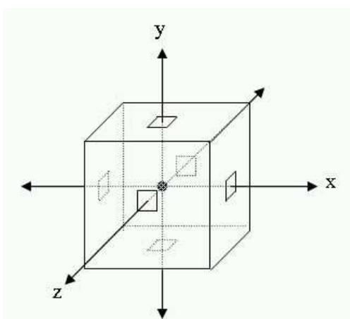
Figure 2: Orientation of the 6 heads of a CSS.
