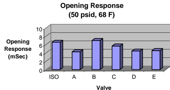
**Figure 12: Opening Response Data****Future MiPS Enhancements**
