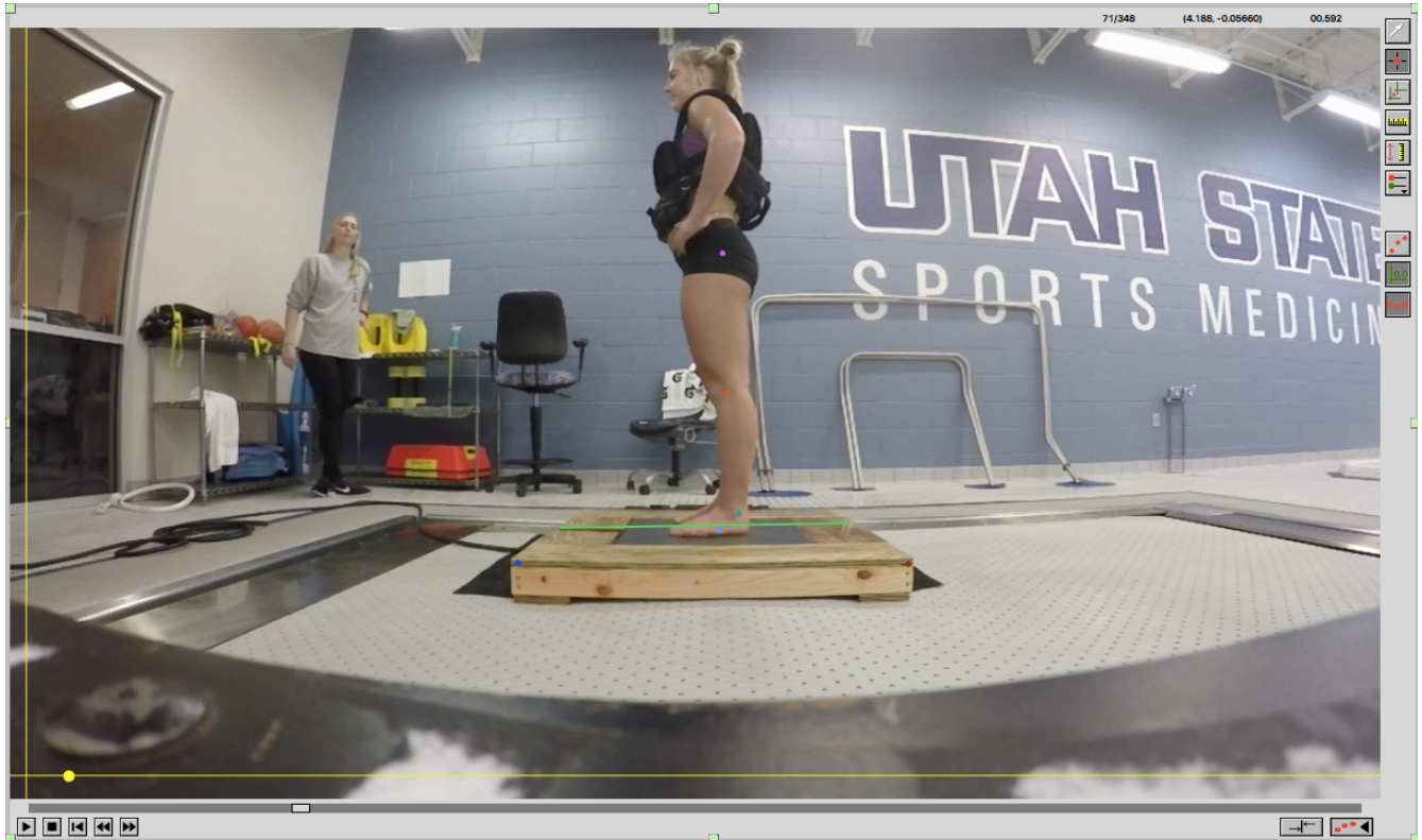
Figure 2: Digitization of anatomical landmarks (colored dots) using LoggerPro software of: 1) greater trochanter of femur (purple) 2) lateral epicondyle of femur (orange) 3) lateral malleolus of fibula (teal) 4) base of the 5 th metatarsal (light blue), with green line representing linear distance reference (9.15 meters) and dark blue/red dots representing horizontal reference.
