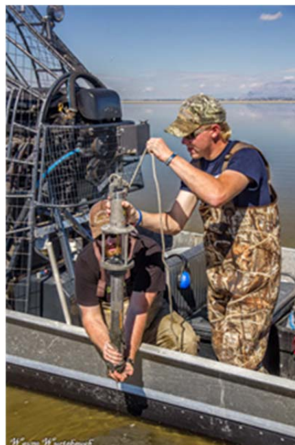
Figure 3: Capping the bottom of the gravity coring device with a stopper on Farmington Bay. Photo courtesy of Wayne Wurtsbaugh.
