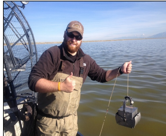
Figure 2. Eckman dredge sampler used in collecting benthic macroinvertebrates.
