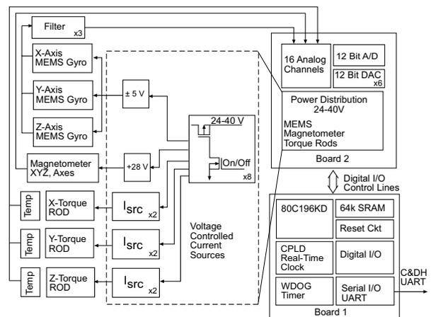
Figure 7. ACS Block Diagram.
