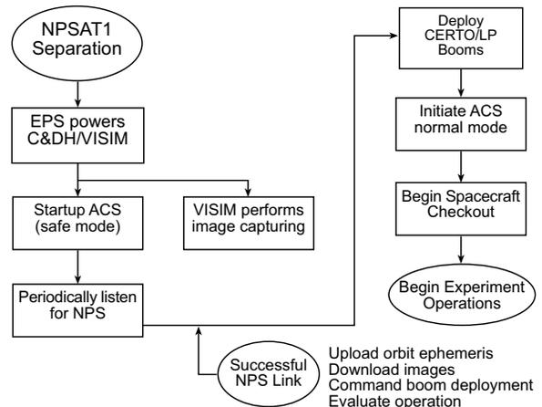
Figure 4. NPSAT1 Startup.
