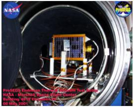
Figure 9 – Icarus in Thermal Vacuum Chamber
