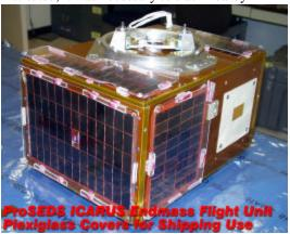
Figure 6 - Endmass View of PAA and Transmitter Antenna with Solar Cell Protective Panels Attached
