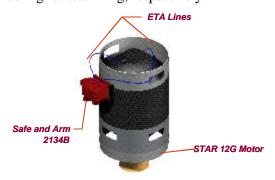
Figure 13. Solid Motor Assembly
