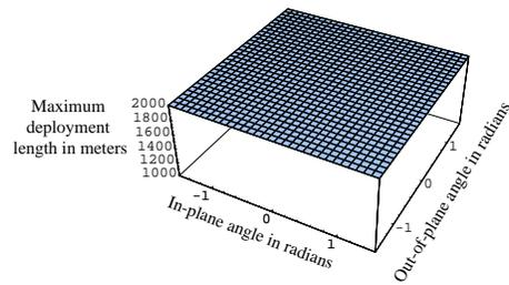
Figure 1: Final Deployed Length as a function of alignment with the local vertical prior to deployment for  $T_0 = 50$  mN,  $m_A = 25$  kg and  $\dot{L}(0) = 5.0$  m/sec.
