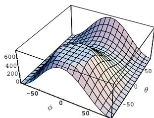
Figure 8: Tension in tether (in Newtons) at end of spin-up (final tether length = 80 meters) vs. initial in-plane ( $\theta$ ) and out-of-plane ( $\phi$ ) angles, assuming  $\theta(0) = \phi(0) = 0$ . Note: Flat region indicates Tension exceeds failure limit of the tether.
