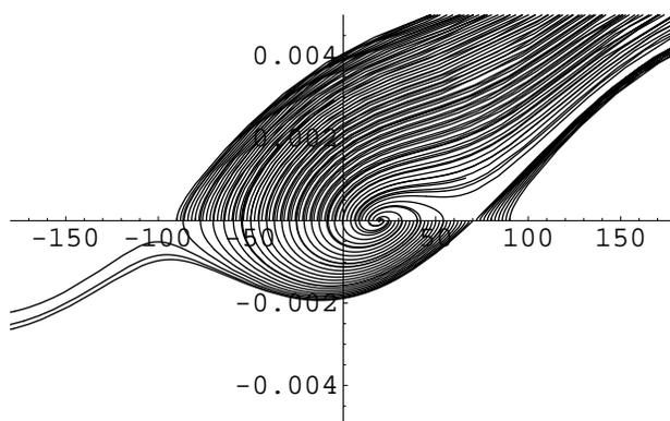
Figure 9: Phase Plane Evolution of  $\theta(t)$  as  $t$  varies from 0 to 5400 seconds;  $\theta_0$  varies from -90 to +90 degrees. ( $\theta$  is plotted on the abscissa and  $\dot{\theta}$  (in radians per second) is plotted on the ordinate).
