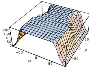
Figure 7: Tension in tether (in Newtons) at end of spin-up (final tether length = 80 meters) vs. initial in-plane ( $\theta$ ) and out-of-plane ( $\phi$ ) angles, assuming  $\theta(0) = \phi(0) = 0$ . Note: Flat region indicates Tension is such that the 25 kg half of satellite experiences at least 1-g of centripetal acceleration.
