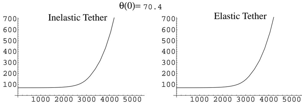
Figure 15: Comparison of Evolution of  $\theta$  with time for models which assume an inelastic tether and an elastic tether, respectively ( $\theta_0 = 70.4$  degrees).  $\theta$  (in degrees) is plotted on the ordinate and time (in seconds) is plotted on the abscissa.
