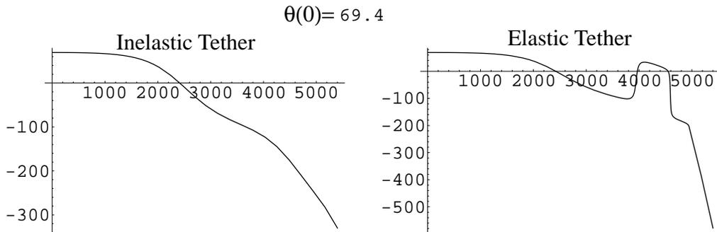
Figure 13: Comparison of Evolution of  $\theta$  with time for models which assume an inelastic tether and an elastic tether, respectively ( $\theta_0 = 69.4$  degrees).  $\theta$  (in degrees) is plotted on the ordinate and time (in seconds) is plotted on the abscissa.
