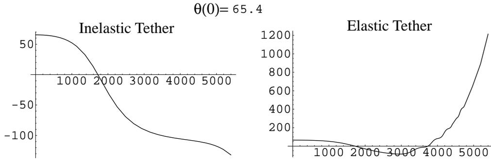
Figure 11: Comparison of Evolution of  $\theta$  with time for models which assume an inelastic tether and an elastic tether, respectively ( $\theta_0 = 65.4$  degrees).  $\theta$  (in degrees) is plotted on the ordinate and time (in seconds) is plotted on the abscissa.
