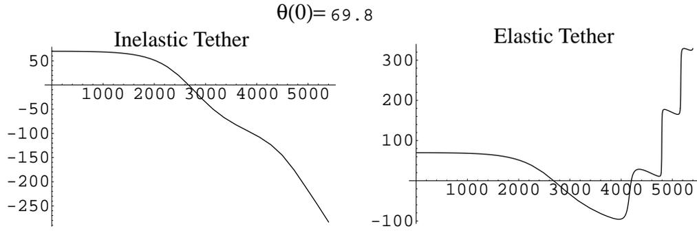
Figure 14: Comparison of Evolution of  $\theta$  with time for models which assume an inelastic tether and an elastic tether, respectively ( $\theta_0 = 69.8$  degrees).  $\theta$  (in degrees) is plotted on the ordinate and time (in seconds) is plotted on the abscissa.
