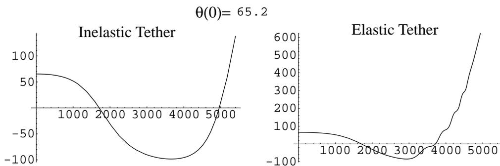
Figure 10: Comparison of Evolution of  $\theta$  with time for models which assume an inelastic tether and an elastic tether, respectively ( $\theta_0 = 65.2$  degrees).  $\theta$  (in degrees) is plotted on the ordinate and time (in seconds) is plotted on the abscissa.
