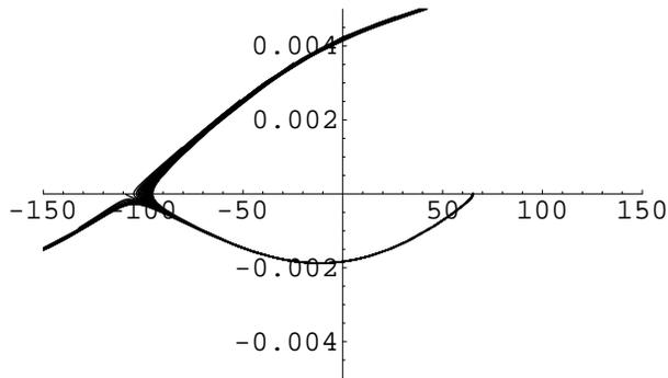
Figure 12: Phase Plane Evolution of  $\theta(t)$  (neglecting tether elasticity) as  $t$  varies from 0 to 5400 seconds;  $\theta_0$  varies from 65 to 65.5 degrees. ( $\theta$  is plotted on the abscissa and  $\dot{\theta}$  (in radians per second) is plotted on the ordinate).
