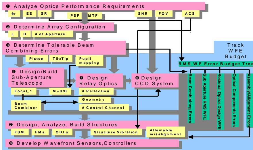
FIG. 3: Sparse-aperture Optics/Control System (SOCS) design flow-down procedures
