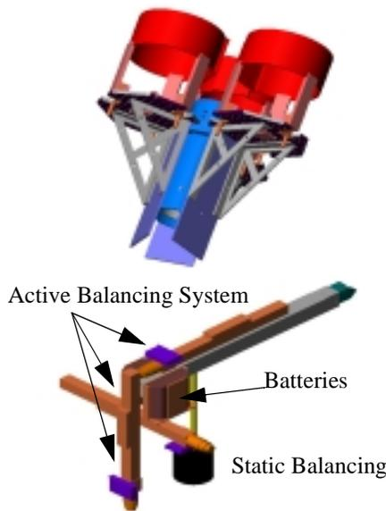
FIG. 21: Assembled aperture mode and swing arm design
