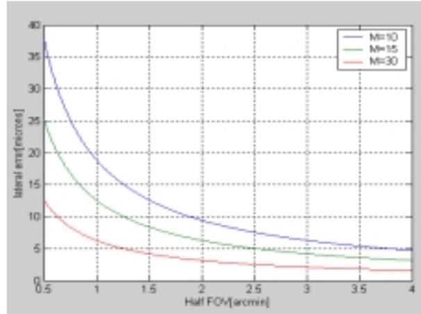
**FIG. 10:** Tolerable pupil mapping error depending on FOV
