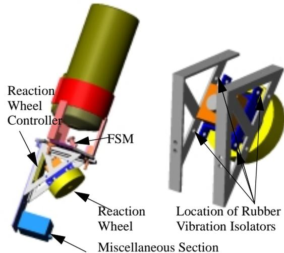
FIG. 19: Aperture module (left) and RWA module (right)
