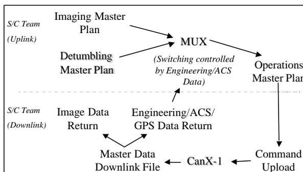
Figure 2: CanX-1 Mission Operation Flowchart
