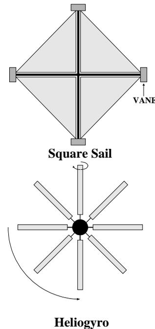
**Figure 7 – Two Main Solar Sail Configurations**
