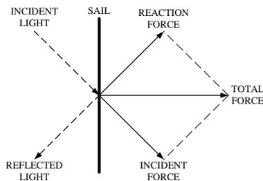
Figure 1 – Forces exerted on Solar Sail due to light [3]
