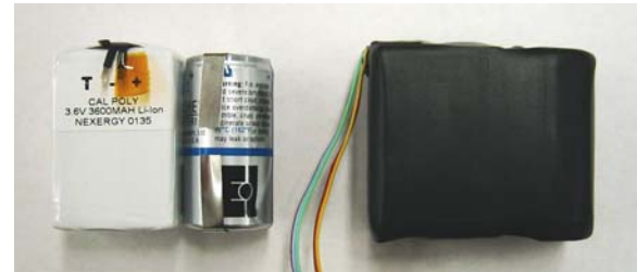
Figure 4.1 – Secondary Battery (left), Primary Cell (center), CP1 Battery Pack (right)
