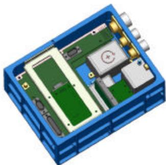
**Figure 2: Avidyne's Guidance, Navigation, and Control System**
