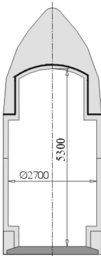
Figure 4. Payload fairing of the Dnepr. Dimensions are in mm. (ISC Kosmotras)
