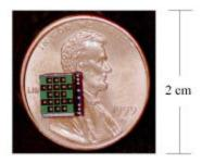
Figure 11: Photo illustrating the size of one of TRW's prototype MEMS propulsion system.
