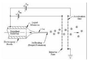
Figure 8: Components of a Colloid thruster. [Figure reproduced from 34]
