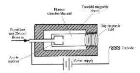
Figure 9: Components of a Hall thruster.
