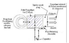
Figure 6: Components of a Pulsed plasma thruster.
