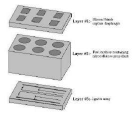
Figure 10: Components of a MEMS thruster array.
