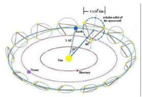
Figure 2: LISA's initial orbit configuration and evolution over 1 year.
