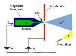
Figure 7: Components of a FEEP thruster.
