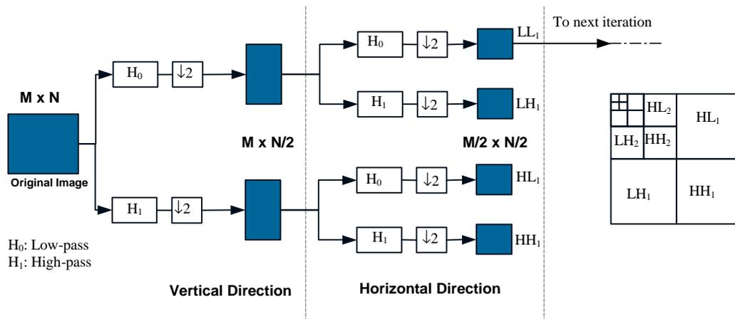
Figure 4. Block Diagram of Discrete Wavelet Transform
