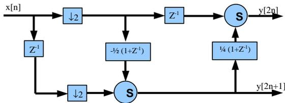
Figure 6. Lifting implementation of the wavelet filter.
