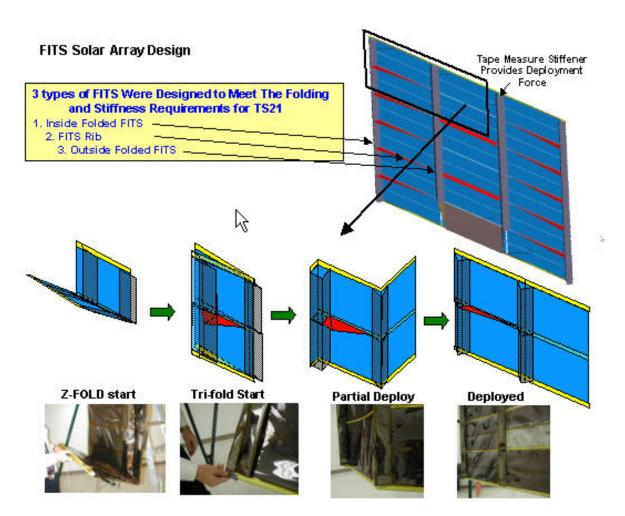
Figure 4. FITS Configuration and Deployment Sequence
