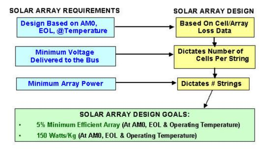
Figure 5. PV Blanket Design Process
