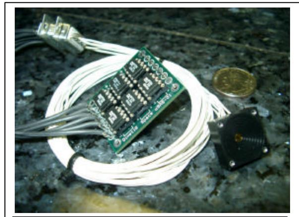
Figure 3: QinetiQ, Ltd. Prototype sensor with electronics board
