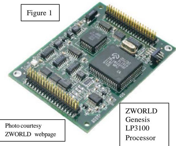
For command and data handling, a ZWORLD Genesis LP3100 (shown in figure 1) was selected as the onboard processor, due to its size (64X89X13 mm), weight and low power consumption (11 to 24 mA). It has 8
