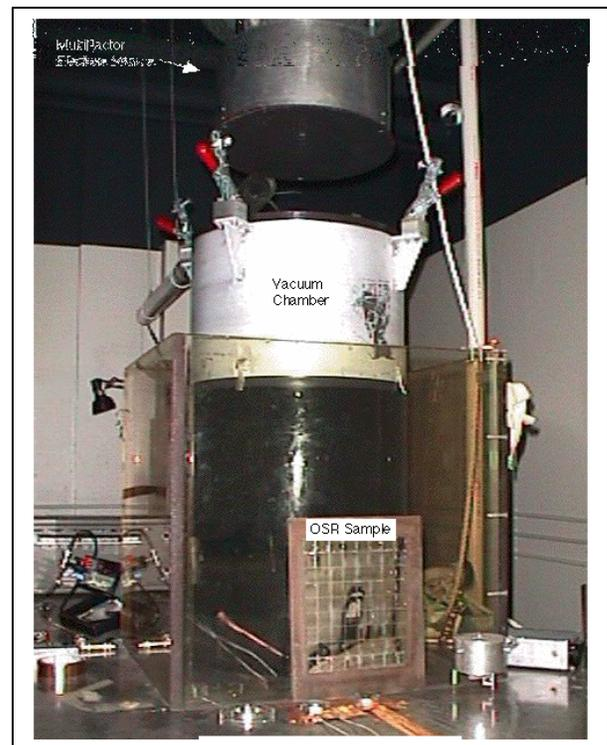
Figure 7: electron beam test chamber at SRI
