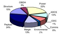
Figure 2 Breakdown of Spacecraft Mass by Subsystem.
