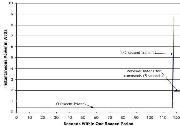
Figure 6) Power profile of the Starshine 3 beacon.
